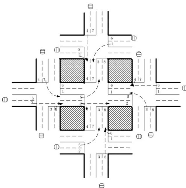
**Figure 1** Five-intersection, centrally connected vehicular traffic network studied
